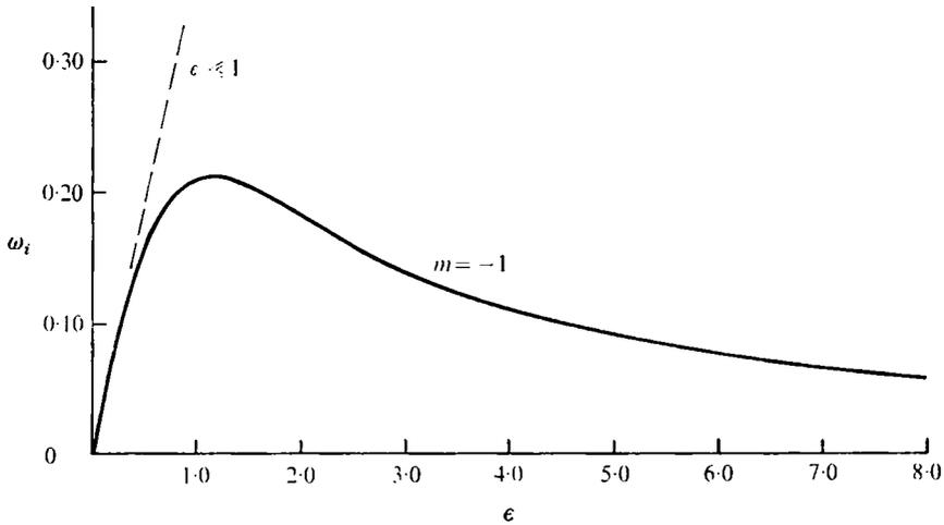
FIGURE 3. Maximum amplification factor *vs.* Rossby number for the sinuous mode,  $m = -1$ .
