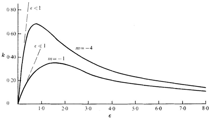
FIGURE 2. Axial wavenumber for fastest-growing waves as a function of Rossby number with  $m = \text{constant}$ .
